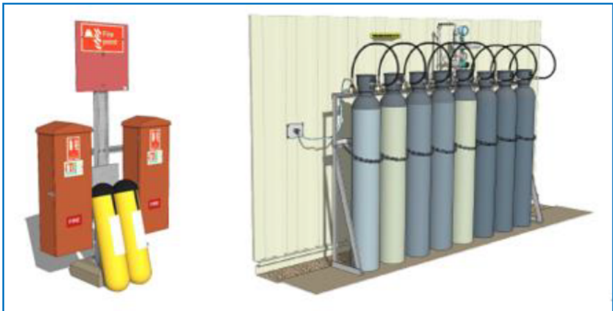
Figure 7: Cabs Fire Suppression (Fire point and Pressurised nitrogen bottles for HI-FOG® system)
